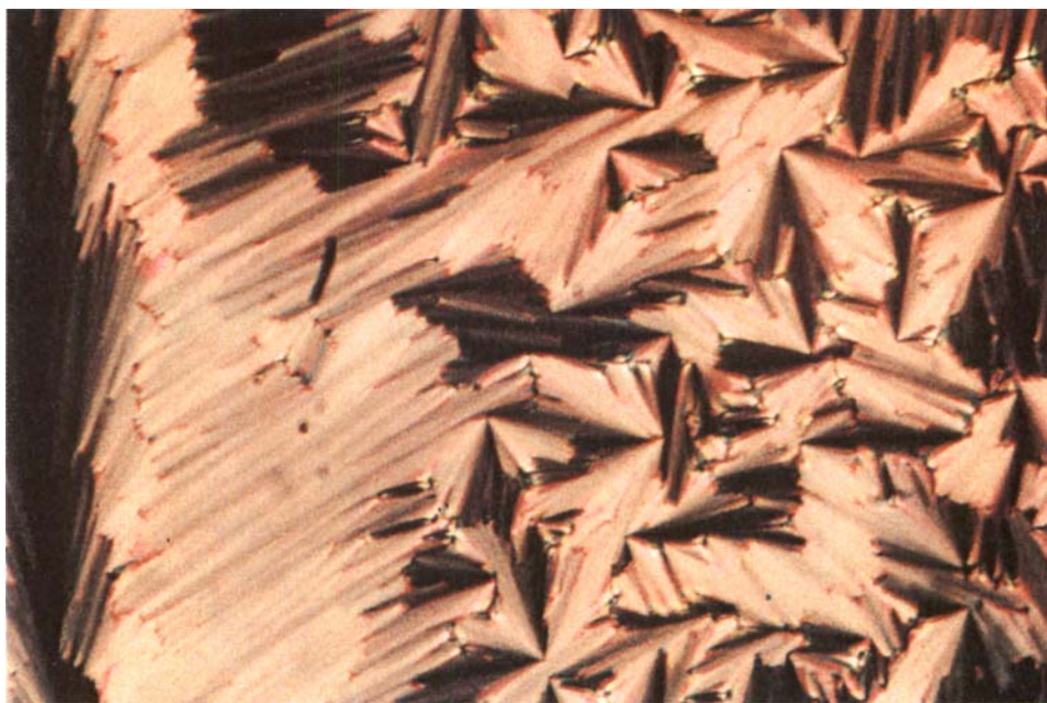
Figure 2. The focal conic fan texture of the S_A phase of 9CT at 117°C. Crossed polarizers. Magnification 200 \times .
